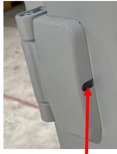
5mm Allen key gives +/- 4mm Lateral Adjustment (ON SIDE OF HINGE) Replace cover caps when adjustment is finished
