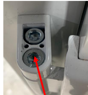
5mm Allen key gives +/- 1mm Compression Adjustment (ON TOP OF HINGE) Replace cover caps when adjustment is finished
